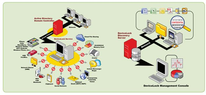
Enterprises can secure any number of remote endpoints with DeviceLock DLP Suite by leveraging its integration with Active Directory and the Windows Group Policy Management Console. DeviceLock Discovery is automatically scanning data residing on network shares, storage systems, and endpoint computers inside and outside of the corporate network
